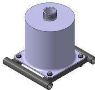
Figure B- 48: Fuel tank mounted to square/rectangular tubes (preferred mounting design)
