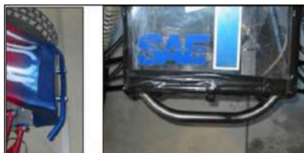
Figure B- 63: Acceptable Front Hitch Point
